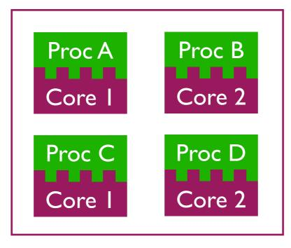
most modern CPUs actually contain multiples CPUs (called "cores") on a single chip
