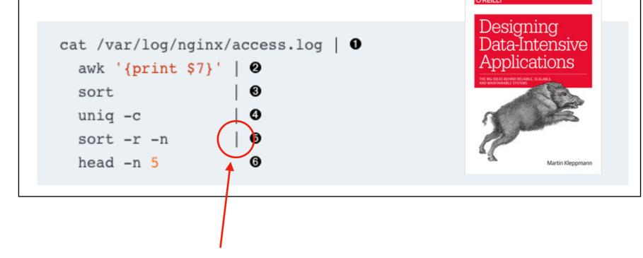
the pipe connects output of one process to input of the next
