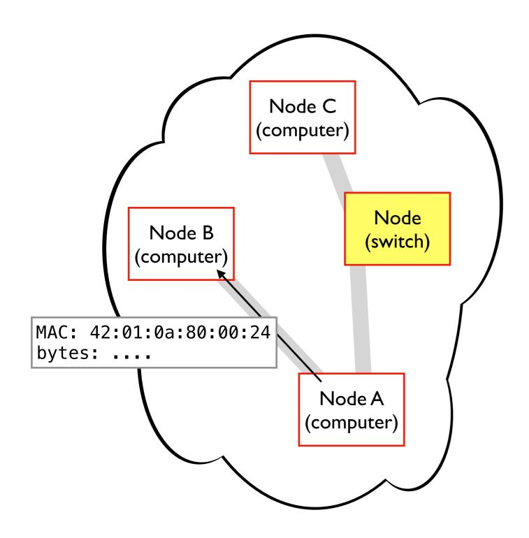
A network has nodes that send bytes to other nodes by MAC address
