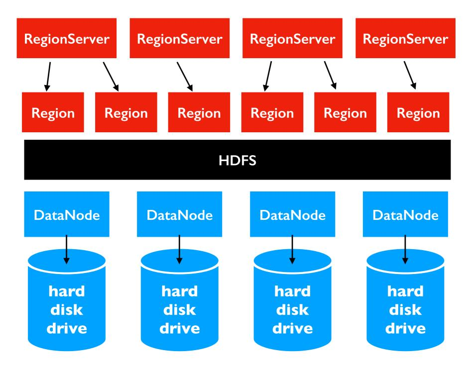
ideally a RegionServer is placed on the same machine as a DataNode holding most of its data
